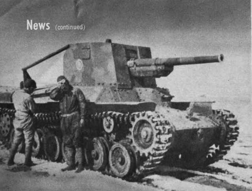
New SP gun is mounted on the Model 97 medium tank chassis. The fighting compartment is set slightly forward of the hull center line.
